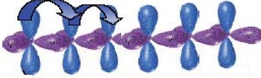
Figure 4.5: The \sigma and \pi orbitals in a chain of carbon atoms. The electrically inert \sigma orbitals, each fully occupied with two electrons (spin up and down) connects the carbon atoms pairwise in the xy plane and they are the reason for the strength of the carbon bonds. The \pi and \pi^* bonds between the p_z are only half occupied. Electrons can therefore hop between the \pi orbitals along the carbon chain, which is the reason for the high conductivity of certain carbon compounds.
